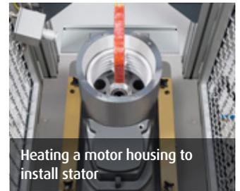
Heating a motor housing to install stator
